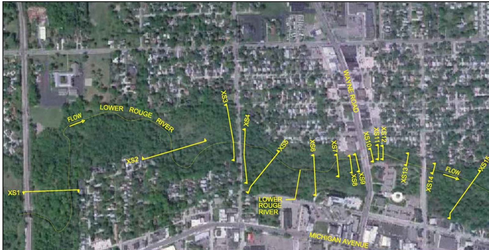
Figure 2. Location of channel cross-sections used to monitor morphological changes in the Lower Rouge River in response to removal of the Wayne Road Dam, Wayne, Michigan.
