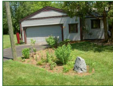
Barbara Burke, Master Composter Farmington Hills Rain water from roof - diverted to rain garden via underground french drain system
